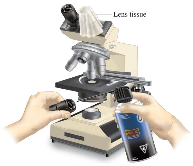
Figure 1.5 When oculars are removed for cleaning, cover the ocular opening with lens tissue. A blast from an air syringe or gas canister removes dust and lint.
